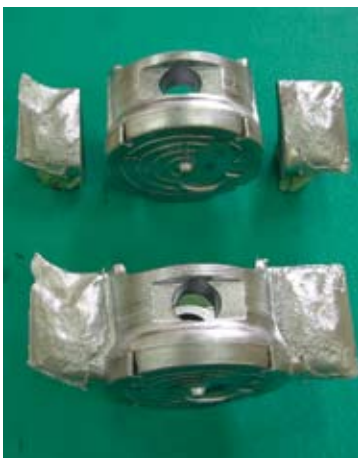
An aluminum piston and the gate. The gate is relatively large compared to the piston itself.
