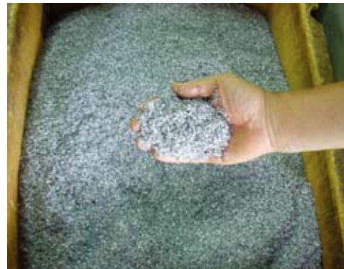
Chips created during cutting are dry.
