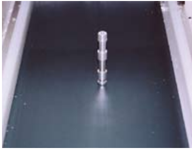
A product is delivered on the clean conveyor without oil stain, which is not expected with oil-based lubricants.
