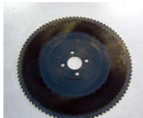
A regrinded metal saw placed on a new metal saw. The metal saw is regrinded until the diameter decreases to \phi 260mm from \phi 300mm and used for about 20 times.
