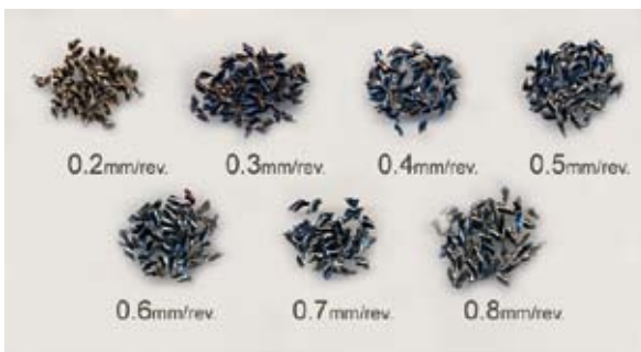
[Pic. 3] A chip shape when feeding of a carbide long drill is changed during near dry machining. Chips are small and curled for every feeding which is a good shape for discharge.
