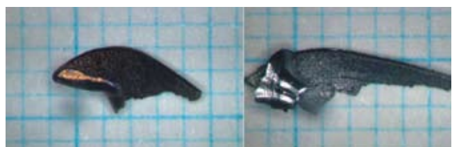
[Pic. 2] Left: near dry machining, right: chips of water-soluble lubricant, provided by FUJIKOSHI
