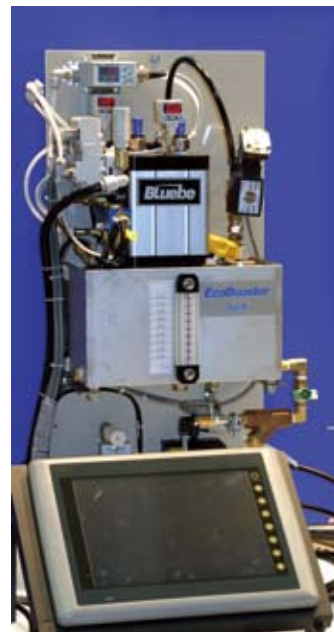
[Pic. 4] A prototype of an inline module exhibited at JIMTOF 2004. The operational status of an applicator is displayed in the panel below.
