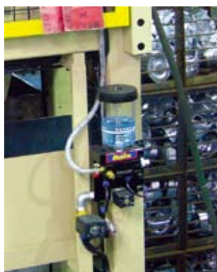
A lubricant applicator for near dry machining installed to the cutting machine. This applicator uses a very limited amount of water-soluble lubricant.
